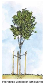
Figure 17.2 Preferred method of staking trees
