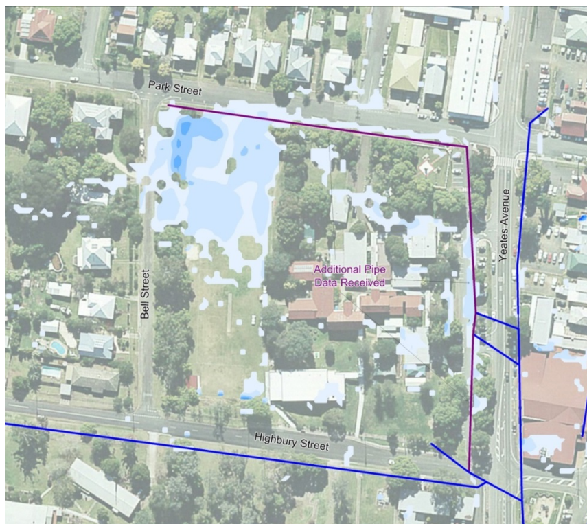
Figure 16 Revised model predictions with missing pipe data included – 10 year ARI flood extent shown
